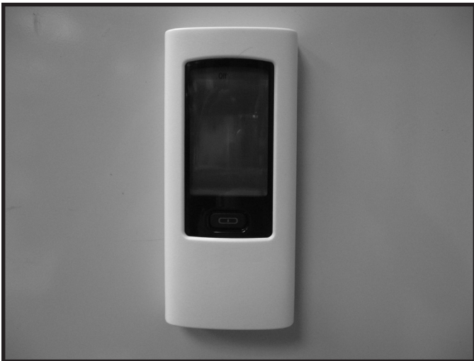
Figure 12.8 Mounting Remote Control Housing
